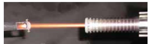
Figure 9: Application of WC-Co-Cr coating with TSR3000H gun to 10 mm internal diameter of a bushing.
