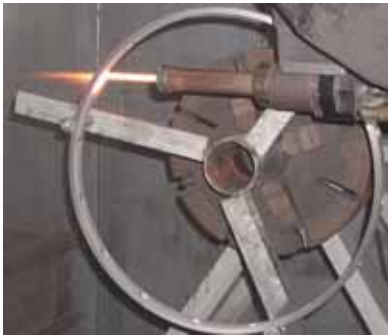
Figure 10: Application of 1.0 mm thick WC-CoCr coating with SB9300 gun on 0.8 m diameter peripheral wall of a jet mill.
