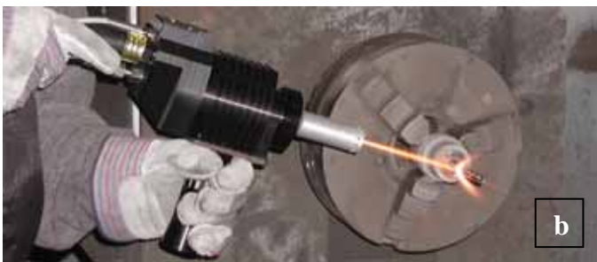
Figure 2: Spraying carbides with SB9300 (a) and TSR3000H (b) guns.
