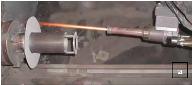
Figure 1: Schematic of the SB9300 gun of the AC-HVAF spray system.
