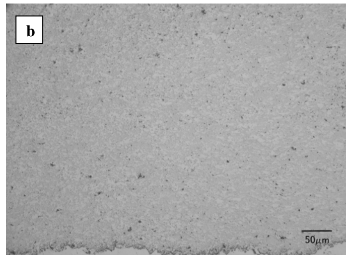
Figure 4: Micrographs of WC-10Co-4Cr coatings applied of agglomerated/sintered (a) and fused/crushed (b) powders; x 200.
